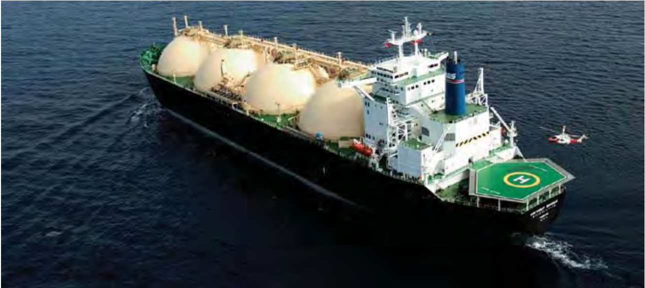
Ships designed especially for storing liquefied gas safely will transport LNG to export markets *
